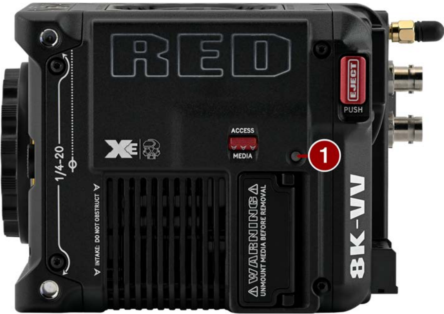
Figure: Camera LED, Left Side
