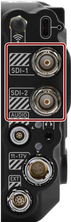
Figure: Front face of the 12G-SDI male BNC connector (looking at the back of the camera).
